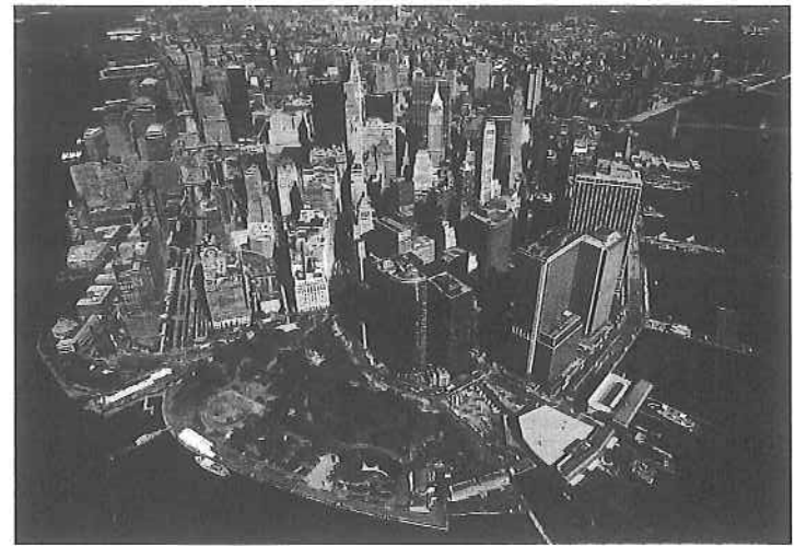
FIGURE 1-10 Changing site of New York City. Much of the southern part of New York City's Manhattan Island was built on landfill. Several times in the past 200 years, the waterfront has been extended into the Hudson and East rivers to provide more land for offices, homes, parks, warehouses, and docks. The World Trade Center was built during the late 1960s and early 1970s partially on landfill in the Hudson River from the colonial era. Battery Park City (at left in the photograph) was built on landfill removed from the World Trade Center construction site. Excavating the landfill from the World Trade Center site unearthed a large number of maritime objects, such as anchors, because the site was underwater in the seventeenth century.
